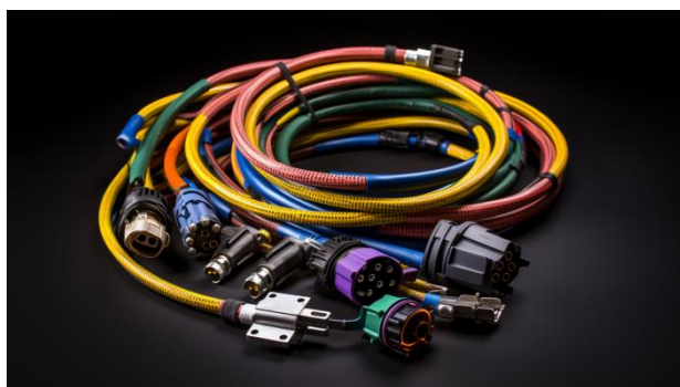
Figure 1. Multifunctional wiring harness with circular and rectangular connectors
