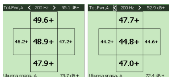
Figure 7. Distribution of sound power over the measurement surfaces at a frequency of 200 Hz, for two different flow rates (left: 5 l/min, right: 15 l/min), obtained using the discrete points method
