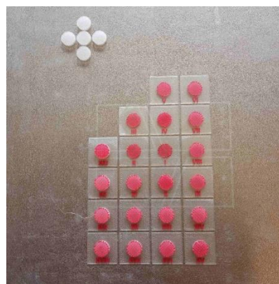
Figure 15. Printing plate; in the top left corner – 5 samples for measuring test with vernier caliper, on the right – layers for Dragonfly model
