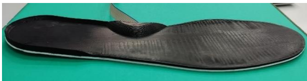
Figure 1. Sensoring insole fabricated from two materials: rigid PLA material (white part), and softer-elastic material TPU (black part)
