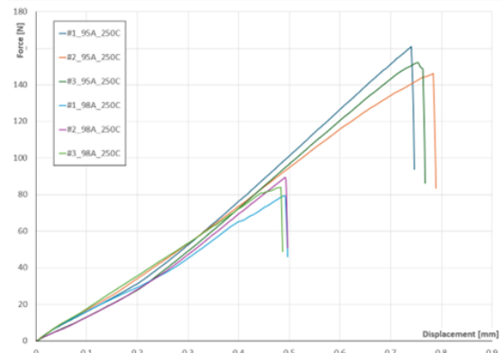
Figure 7. Diagram tensile test for determination of the maximal force for layer separation for temperature 250°C
