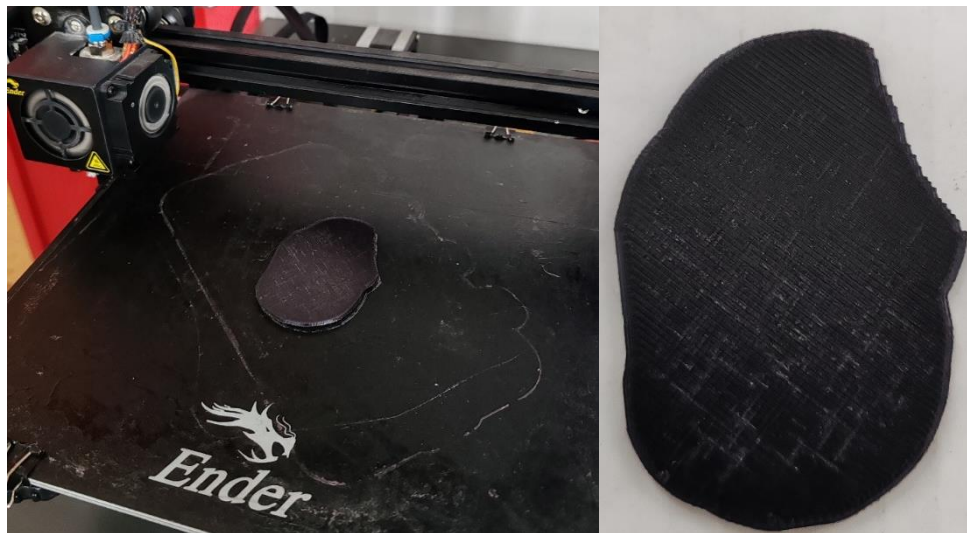
Figure 6. The FDM printing process and Physical nylon model of personalized wound dressing cover
