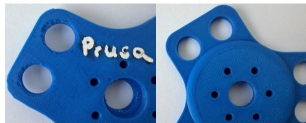
Figure 6. Surface finish obtained using PrusaSlicer
