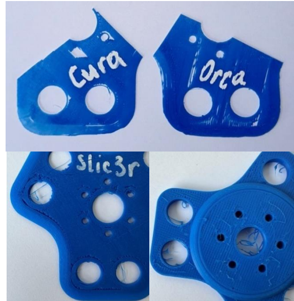
Figure 5. Printing defects observed when using Cura, Orca, and Slic3r slicers
