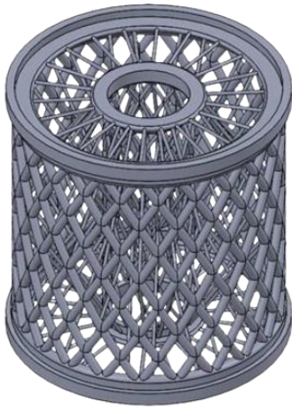
Figure 2. Custom lattice like scaffold
