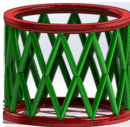
Figure 2. Lattice like scaffold
