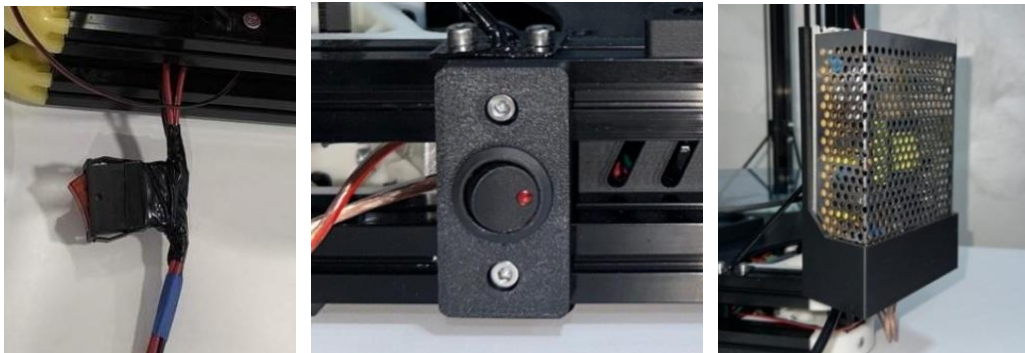
Figure 15. The initial power switch and the designed power switch and power supply housings
