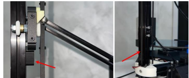
Figure 19. Mechanical stoppers (left) and cable covers (right)
