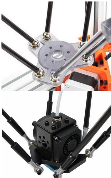
Figure 3. Different types of joints in Delta printer variations
