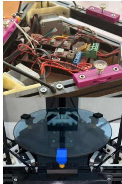
Figure 12. The original and improved bed leveling system
