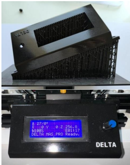
Figure 17. Housing after printing and final assembled part
