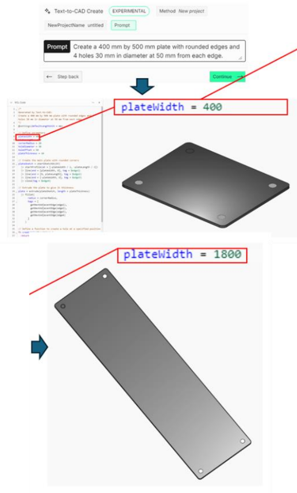
Figure 9. Parametric CAD model created based on text prompt in Zoo Design Studio
