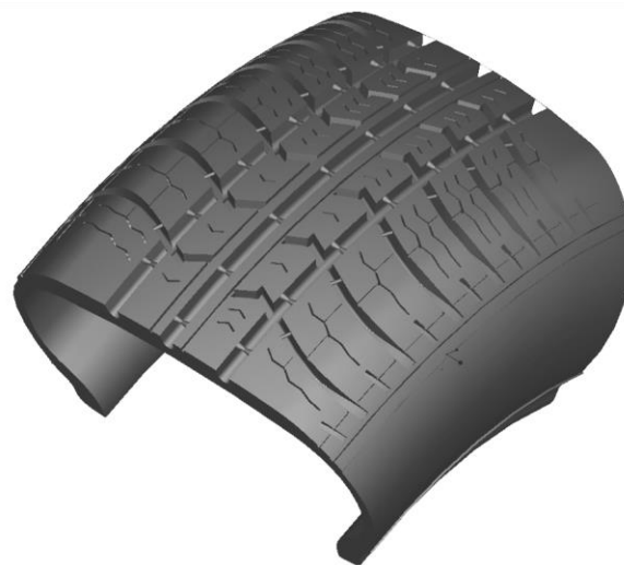
Figure 2. A parametric feature-based model of pneumatic tire created in Pro/ENGINEER [9]
