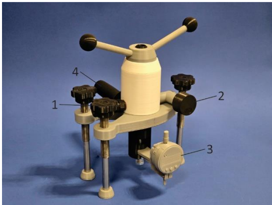
Figure 9. The third iteration of the prototype device for testing anchor bolts (1 - wireless pressure sensor; 2 - analog pressure gauge; 3 - wireless displacement sensor; 4 - handle for carrying the device)
