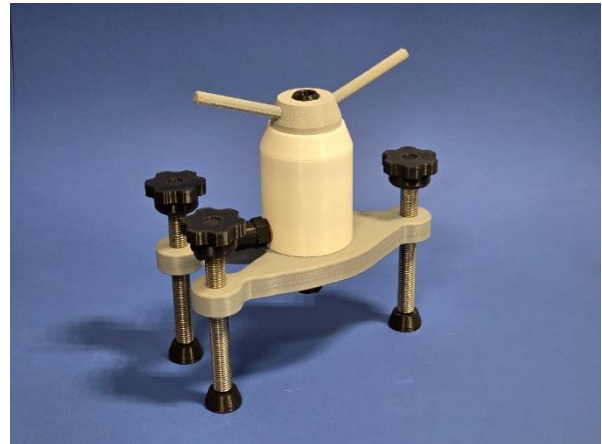
Figure 8. The Iteration 2 of the prototype anchor bolt testing device
