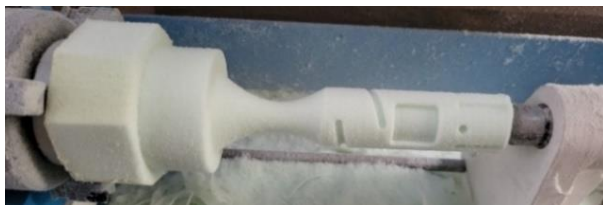
Figure 7. Example machining workpiece which is programmed using CAD/CAM system
