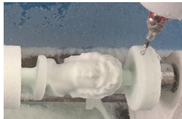
Figure 8. Example machining workpiece which is programmed using Vectric Aspire
