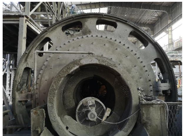
Figure 4. Industrial gear with 3,5 m diameter used in copper mining industry
