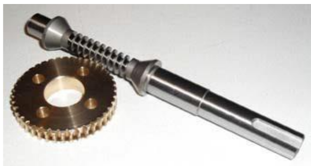
Figure 2. Worm gear set with center distance 30 mm in which worm gear is made from bronze
