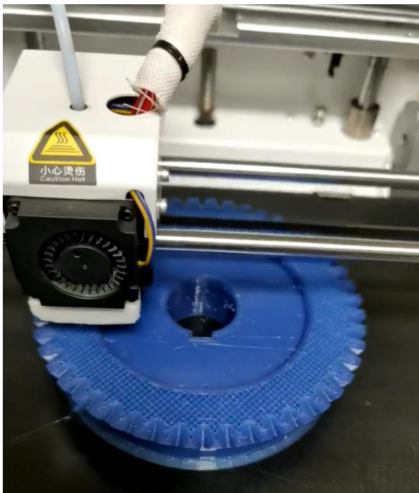
Figure 3. FDM 3D printing of bevel gear
