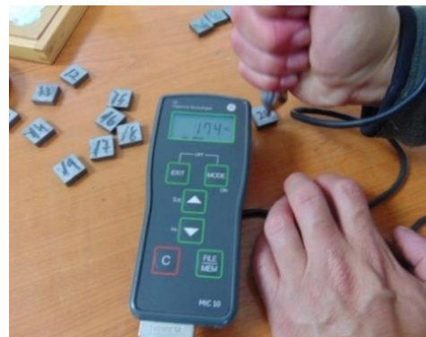
Figure 3. Portable KrautKramer MIC 10 device used for hardness measurement.
