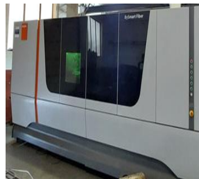
Figure 1. BySmart Fiber Bystronic laser cutting machine used in the experiments.
