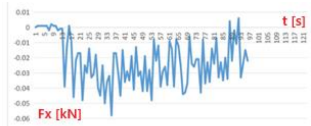
Figure 8 F_x component of the cutting force, with v_f up direction ( D5; z2; a_e5; a_p0,5 )
