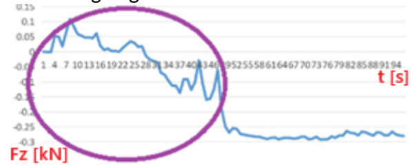
Figure 12 F_z component of the cutting force (D5; n400; z2; a_e 5; a_p 3,5)
