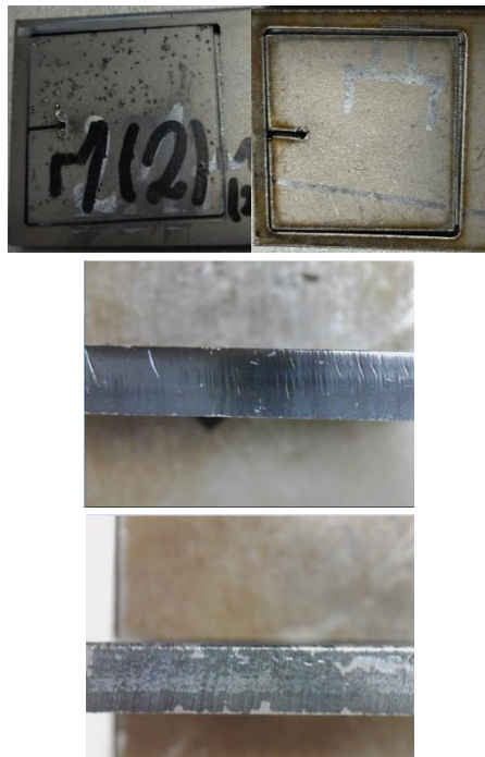
Figure 9. Sample 21, the upper and bottom side and the cut surfaces
