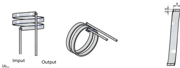
Figure 2. Schematic geometry of the spiral cooling jacket
