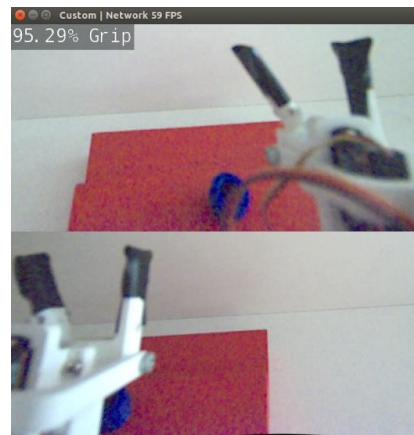
Figure 13. Mobile robot's view of the scene and gripping accuracy prediction.
