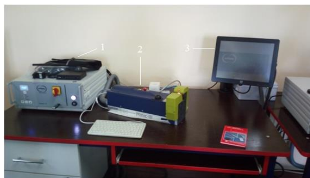
Figure 3. Ultrasonic welding machine: 1- ultrasonic generator, 2- welding device, 3- display
