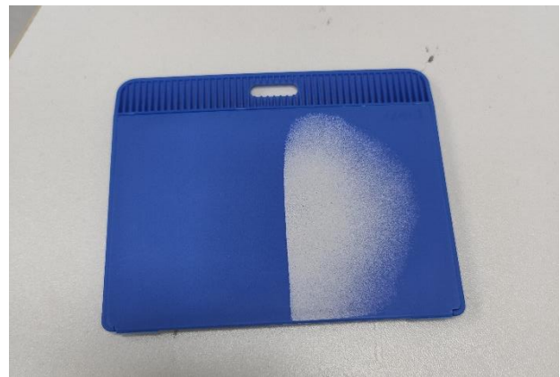
Figure 3. AESUB blue scanning spray layer applied on plastic card.
