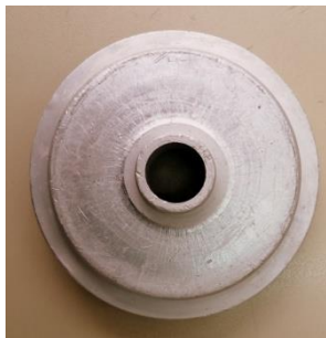
Slika 3. Aluminium piston (final shape after machining)
