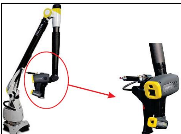
Figure 3. MMDx100 laser scanner integrated with Nikon MCAx+2.0 measuring arm
