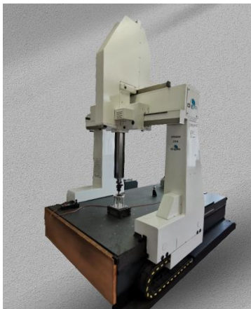
Figure 1. Real measuring machine DEA Epsilon 2304. - Physical twin
