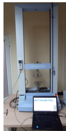
Figure 3 Shimadzu Table-top AGS-X 10kN universal testing machine
