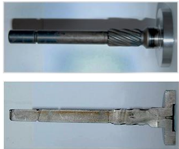
Figure 6. Heat treated shaft (above). Longitudinal cross-section of the planetary shaft (below). Cutting was made with water jet cutting machine. Thickness of hardened case is approximately 1.4 mm
