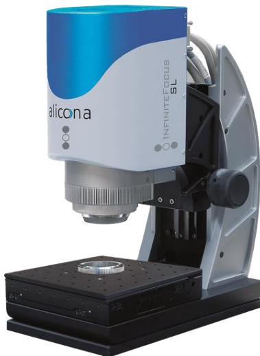
Figure 2. Infinite Focus SL focus variation measuring device [15].
