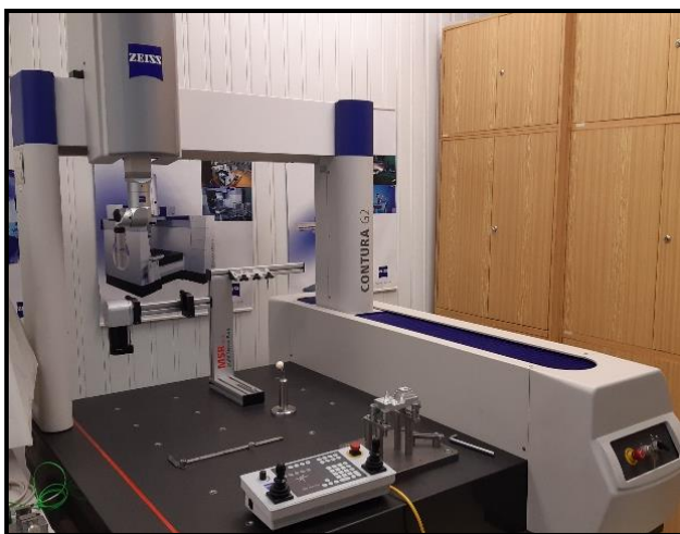
Figure 2. Coordinate measuring machine Carl Zeiss Contura G2 RDS
