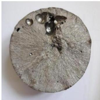
**Figure 6.** Casting part - flotation ball after impact testing
