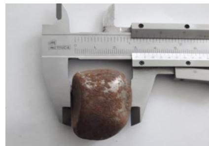
**Figure 9.** Flotation ball wear level
