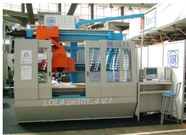
**Figure 11.** Vertical 3-axis parallel kinematics milling machine
