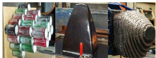
**Figure 14.** The impact attenuator made of tin cans and pu foam (left), ABS plastic (middle) and comb shaped Al slab
