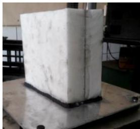
**Figure 9.** The impact attenuator made of ROHACELL foam
