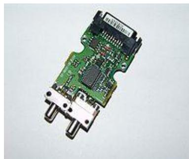
**Figure 15.** Network card for fiber communication
