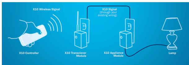
**Figure 2.** How X10 technology works
