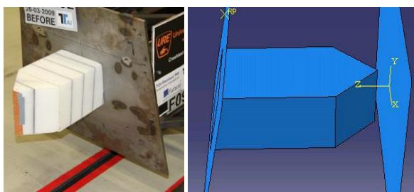
**Figure 7.** Attenuator before „crush“ test (left) and Abaqus model (right)
