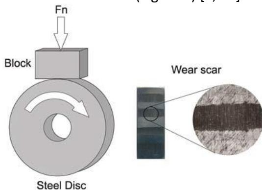
**Figure 2.** Method BLOCK-ON-DISC for testing coefficient friction and wear volume [10]
