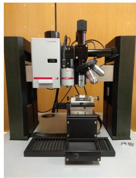
**Figure 2.** CSM (Anton Paar) Micro Scratch Tester (MST)
